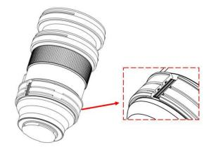
Insert the plastic C-ring for zoom gear as shown and place it over the lens
