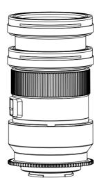
The tightness between the both gears and the lens can be adjusted by removing or adding rubber grips on either sides of the plastic C-ring, spare rubber grips are included in the package.
