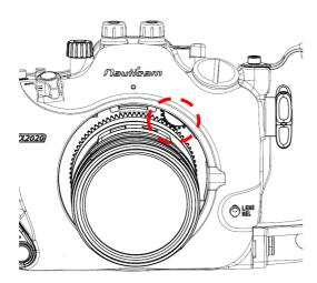
The SSF2470-Z Zoom Gear can be controlled by zoom/focus knob of the housing.
